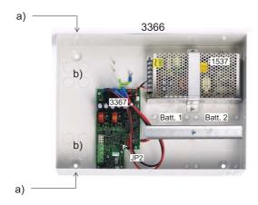
External power supply (3366) inside view: <u>Rectifier</u> 230 V AC / 24 V DC (1537), <u>Charger board</u> (3367) and space for two <u>batteries</u> rated 12 V / 6.5-7.5 Ah (size 150 x 65 x 94 mm).
