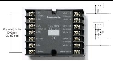
**VO0 & VO1**: **AD**=Alarm Device (bell, siren, etc.). **VO2**: **M**=Fire door release magnet(s). **D1**=Protective diode (e.g. 1N4004), when required. **D2**=Series diode (e.g. 1N4004). **C** (470nF), to be connected in the last device <u>or</u> in up to five devices.
