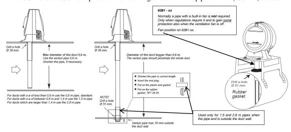
*Left:* How to suit the pipe to different widths of the ventilation duct. 6377 can be mounted vertical on the duct and 3 x the duct diameter <u>before</u> or 5 x the duct diameter <u>after</u> a disturbance, i.e. a fan, a bend, a filter, a silencer, a damper, etc.
