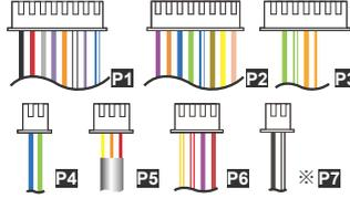
※ P7 only provide to the controller that have doorbell function.
