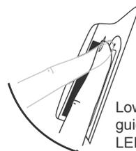
Lower the finger down along the finger guide slowly. Release the finger when red LED turns off.
