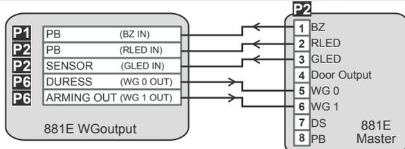
1. When AR-881EF/V become WG mode, it can be used with any controllers.
